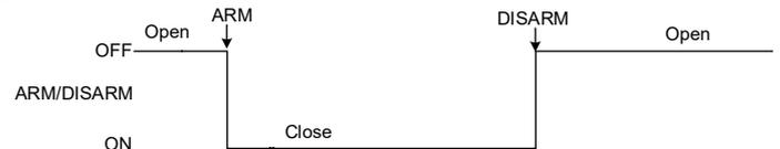
**Buzzer:** Output for connection of audio indicator. After the alarm system activated a pulse signal is generated within Exit Delay time, and continuous signal - within Entry Delay time or when the alarm system is disturbed. When the alarm system is turned off, operates like keyboard buzzer.
